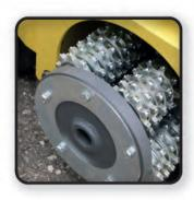
The rotating steel drum generates centrifugal force thus throwing the tungsten-pointed, heattreated steel cutter at the surface to be prepared or corrected.
