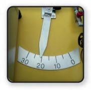
Cutting depth indicator clearly shows depth of cutters in the cut.
